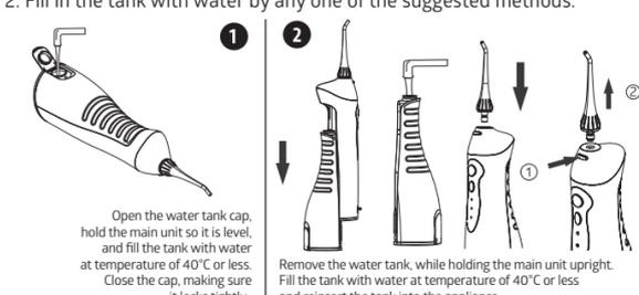
**ⓘ CAUTION!** Never use a water-filled irrigator without the nozzle, which may cause device malfunction.
