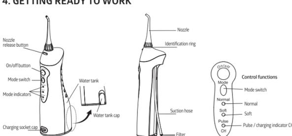
Press On/off button to switch the appliance on/off. Press Mode button to select the desired water jet mode (normal, soft, pulse). The mode selected will be shown by the mode indicator. If you want to use a different mode, press the mode switch until it changes to the desired setting. Pressing the mode switch will change the mode from Normal to Soft and Pulse.
