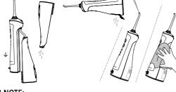
Always drain the remaining water. This will help prevent contamination and growth of bacteria in water that remained in the device.
